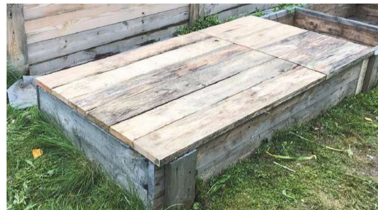
Figure 5 – Construction of the wooden box for studying MSW biodegradation
