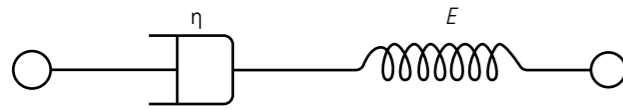
Figure 4 – Maxwell model for a visco-elastic damper. The viscous damper is connected in series with an elastic spring
