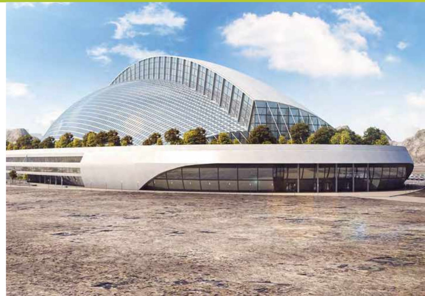
Figure 16 – Rendering of the ECH-Earth (option) with a structural solution in the form of a torus fragment with a longitudinal section and a risen part of roofing
