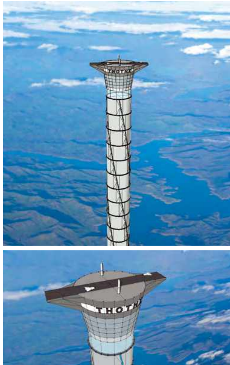
Figure 5 – Diagram of Thoth Technology inflatable elevator
