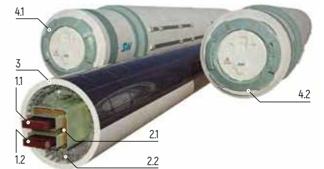
Figure 4 – GPV construction (option): belt flywheels 1.1 and 1.2, placed in vacuum channels; drive systems 2.1 and 2.2, located inside the body 3; external compartments of the capsule 4: passenger 4.1 and cargo 4.2 (visualization)
