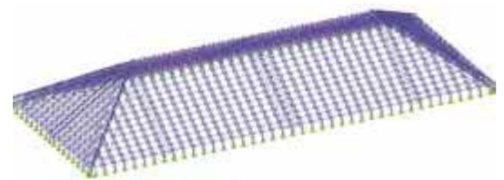
Figure 10 – An option of the structural solution for the ECH-Earth in the form of a pyramid, rectangular in plan
