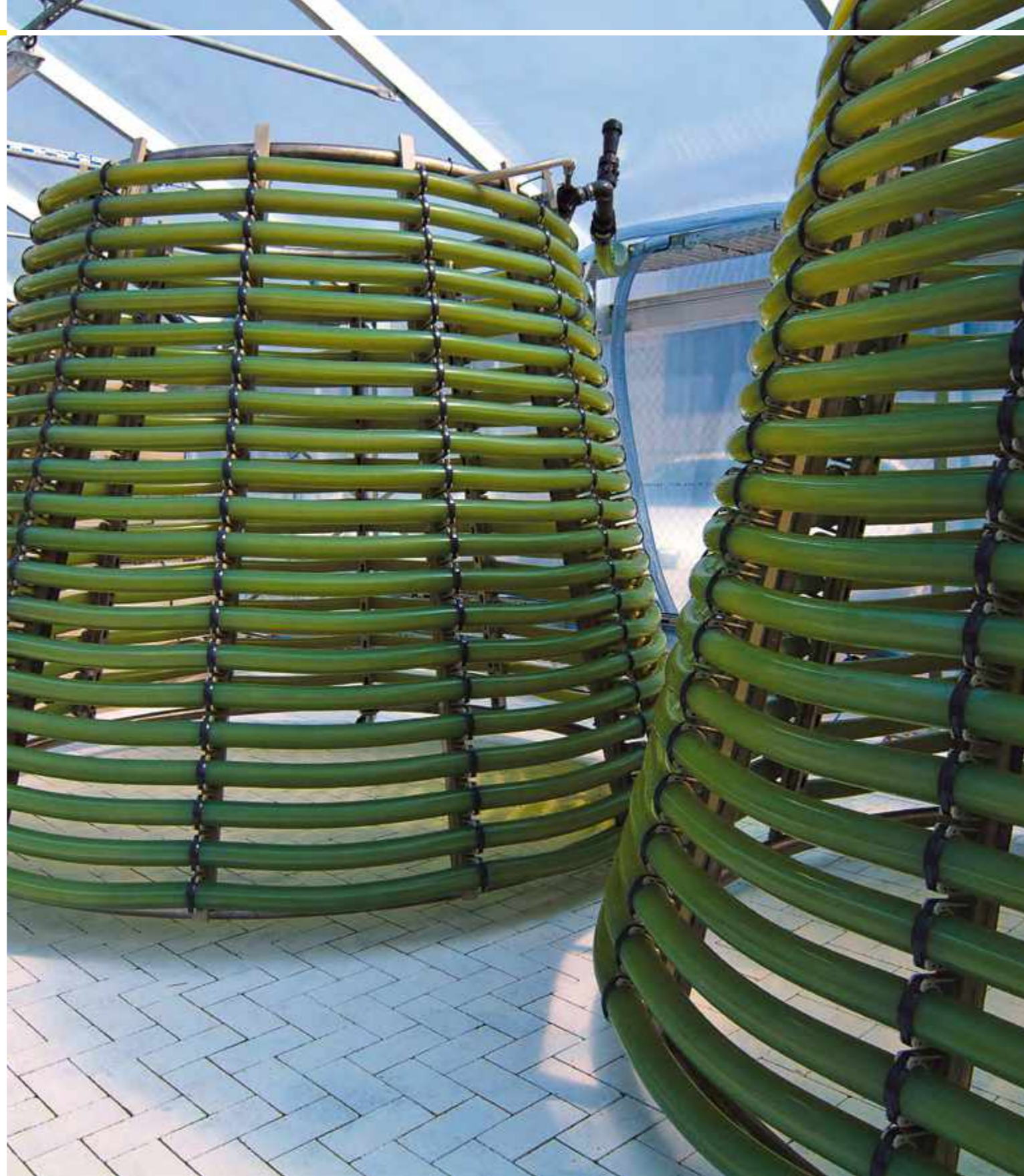
Figure 6 – Photobioreactor for closed-type chlorella cultivation
