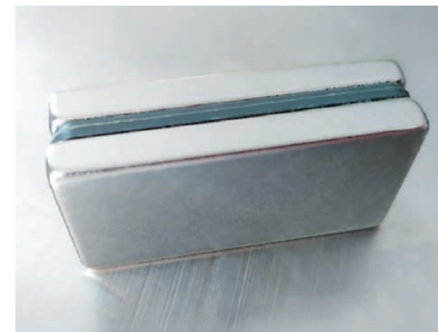
Figure 1 – Magnets N40 ( \text{Nd}_2\text{Fe}_{14}\text{B} ) of the size 40 \times 20 \times 5 mm
