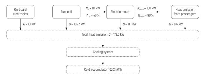
Figure 4 - Flows of excess thermal energy of the HV and their estimated capacity
