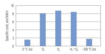
Figure 6 – Specific cost of the refrigerants per 1 kW·h of electrical energy consumption per one HV trip
