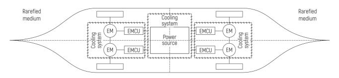
Figure 1 – Diagram of the HV power plant: EM – electric motor; EMCU – electric motor control unit
