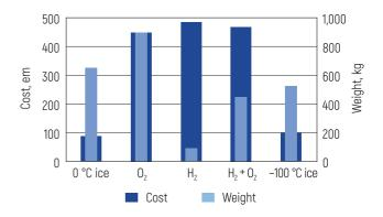
Figure 5 – Cost and weight of the refrigerants in the battery per one HV trip
