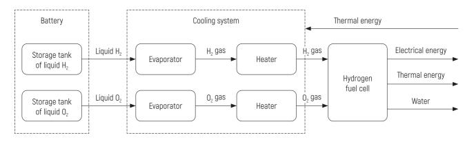
Figure 2 - Diagram of the use of hydrogen and oxygen as a refrigerant and energy sources on board the HV
