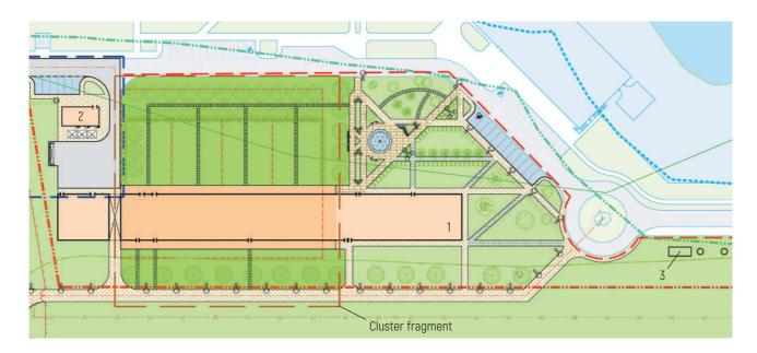
Figure 9 – Layout of a multifunctional building on the territory of the Unitsky's Farm Enterprise (variant): 1 – multifunctional building; 2 – boiler room; 3 – wastewater treatment unit
