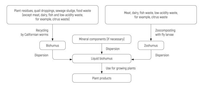
Figure 15 - Diagram of processing solid food waste to obtain plant products
