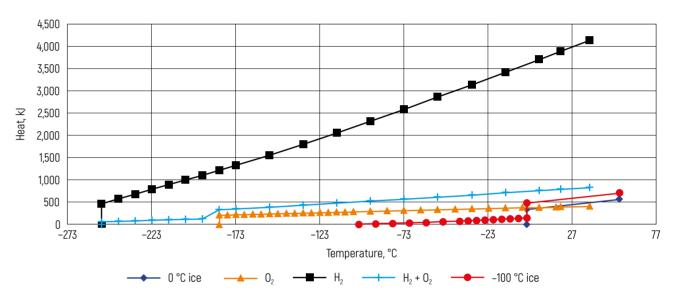
Figure 3 - Dependence of heat absorbed by the refrigerant on temperature
