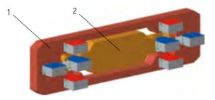
Figure 6 - Magnetic cluster: 1 - stator; 2 - rotor
