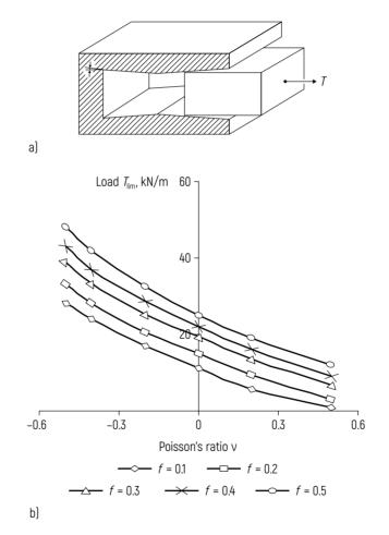
Figure 3 – Frictional behavior of auxetics: a – structure of the friction joint; b – dependence of the limiting shear load on the Poisson's ratio v at different coefficients of friction
