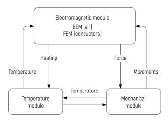
Figure 3 – Diagram for modeling a connected problem: electromagnetic – mechanical – thermal interaction
