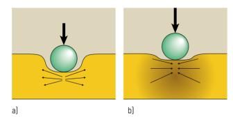
Figure 2 – Behavior during indentation material [14]: a – conventional material; b – auxetic
