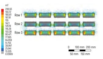
Figure 15 – Change in the distribution of the magnetic field density of the system when the gravity force of the Earth at its surface acts on the rotor (view in the X axis direction based on Figure 7)
