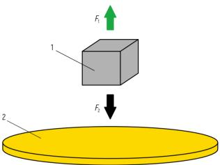
$<sup>\</sup>label{eq:Figure 3} \begin{array}{l} \mbox{Figure 3} - \mbox{Levitation over a superconductor:} \\ \mbox{1 - permanent magnet Nd}_2\mbox{Fe}_{14}\mbox{B; 2 - ceramic disc YBa}_2\mbox{Cu}_3\mbox{O}_7 \end{array}$
