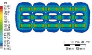
Figure 9 – Magnetic induction lines of the system (view in the *X* axis direction based on Figure 7)
