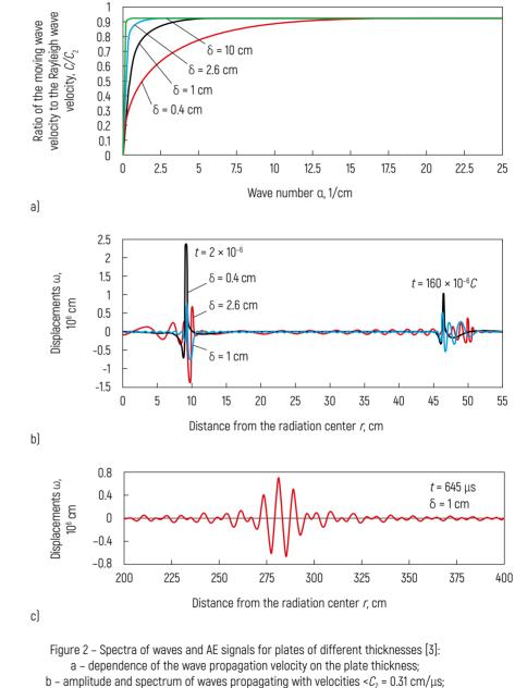
wave propagates with a velocity of  $0.927C_2$ , which is close to the Rayleigh one in terms of properties. As follows from the obtained dependence of the wave amplitude on the thickness of the plate and the distance from the place of radiation (Figures 2b, 2c), a source of the same power generates more significant wave amplitudes in a thin plate than in a thick one. This is how it can be explained that the radiation energy is absorbed faster in a larger volume of metal.
