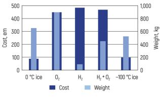
Figure 5 - Cost and weight of the refrigerants in the battery per one HV trip
