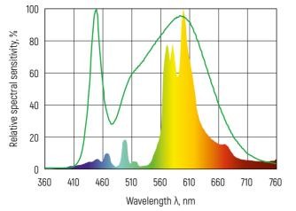
Figure 4 – Comparison of the spectral composition of the radiation of a typical HPS 1000 lamp and a typical LED (green line)
