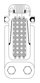
Figure 3 - Rail of the track structure, the running track of which is made up of vertical steel plates mounted in parallel on an edge
