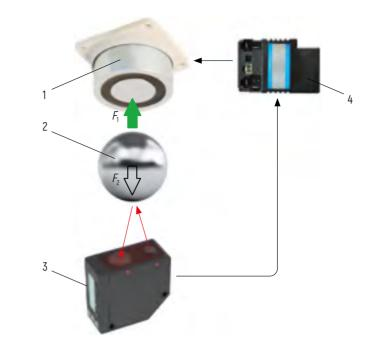
Figure 1 – Electromagnetic levitation: 1 – electromagnet; 2 – levitating body; 3 – distance sensor; 4 – control unit
