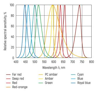
Figure 3 – Typical spectra of colored LED lamps
