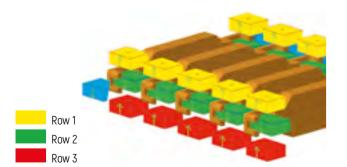
Figure 13 – Rows of rotor magnets (row 2) and stator magnets (rows 1 and 3)
