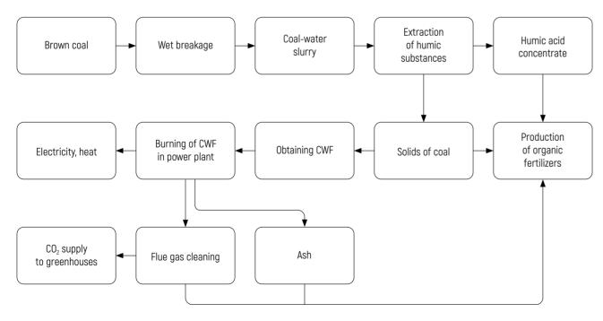
Figure 4 – Integrated (waste-free) use of brown coal
