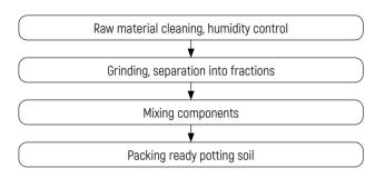
Figure 4 – Technological chain of classic potting soils production
