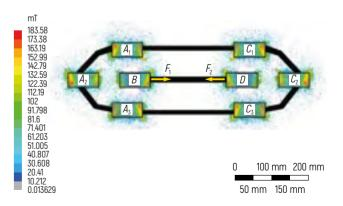
Figure 11 – Forces acting in the X axis direction from the stator side
