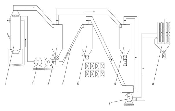
Figure 6 – Perlite production process flow diagram: 1 – shaft expansion furnace; 2 – air supply fan; 3, 5, 6 – cyclones; 4 – additional path of pneumatic transport; 7 – smoke exhauster; 8 – bag filter
