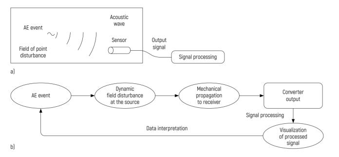
Figure 1 - AE signal analysis circuit: a - schematic diagram; b - general algorithm of functioning
