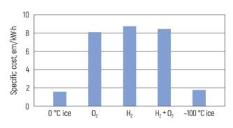
Figure 6 - Specific cost of the refrigerants per 1 kW·h of electrical energy consumption per one HV trip
