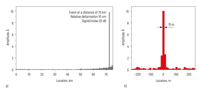
Figure 5 - Sensitivity of the DAS method in relation to an event located at a considerable distance: a - registration; b - spatial resolution
