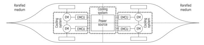
Figure 1 - Diagram of the HV power plant: EM - electric motor: EMCU - electric motor control unit
