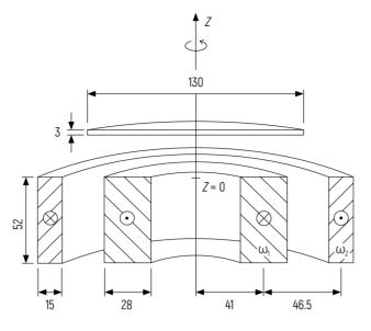
Figure 5 – Dimensions of the electromagnetic levitation device of the round plate, mm
