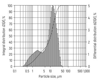
Figure 7 - Fractional composition of crushed brown coal
