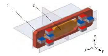
Figure 7 - Rotor freedom degrees: 1 - stator; 2 - rotor
