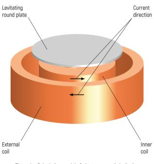
Figure 4 – Calculation model of electromagnetic levitation of the round plate
