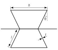
Figure 7 – Elementary cell of a honeycomb-like structure with a negative Poisson's ratio
