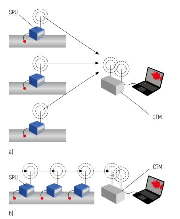
Figure 7 - Intelligent diagnostic system: a - direct signal transmission mode; b - network mode
