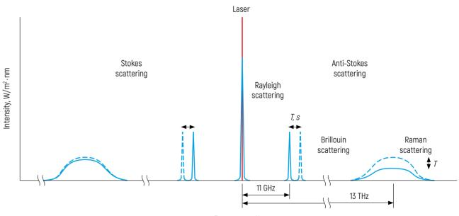
Figure 4 - Schematic representation of the spectral components of light scattering in an optical fiber
