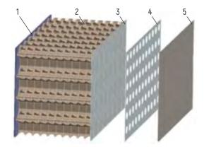
Figure 9 – Perspective view of the structure design of the ECH shell: 1 – outer shell plating; 2 – plastic dampers in the form of interference tunnels; 3 – vacuum insulator; 4 – interference grating; 5 – soil surface [36]
