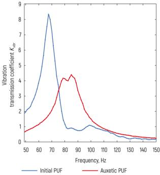
Figure 4 – Vibration transmission coefficients  $K_{\rm vibr}$  of initial and auxetic PUF at small excitation amplitudes [20]
