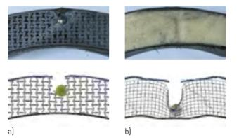
Figure 6 – Experiment and finite element modeling. Pulse effect on a sandwich panel with filler: a – auxetic honeycomb-like material made of PLA-plastic; b – conventional PUF [32]
