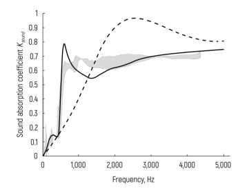
Figure 5 – Sound absorption coefficients  $K_{sound}$  of samples with a thickness of 26 mm [31]
