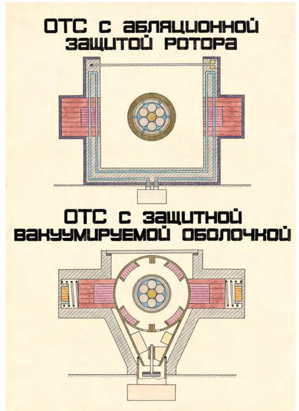
UPT with ablative protection of the rotor and UPT with vacuum protective shell. 1974
