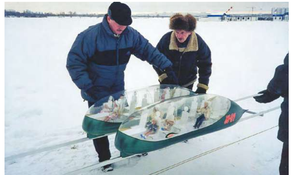
First test of a double-rail track and a double-body unibus model (scale 1 : 5). Tushino airfield, December 2000
