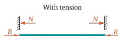
The beam is not subject to compressive buckling (at N \geq R ).
