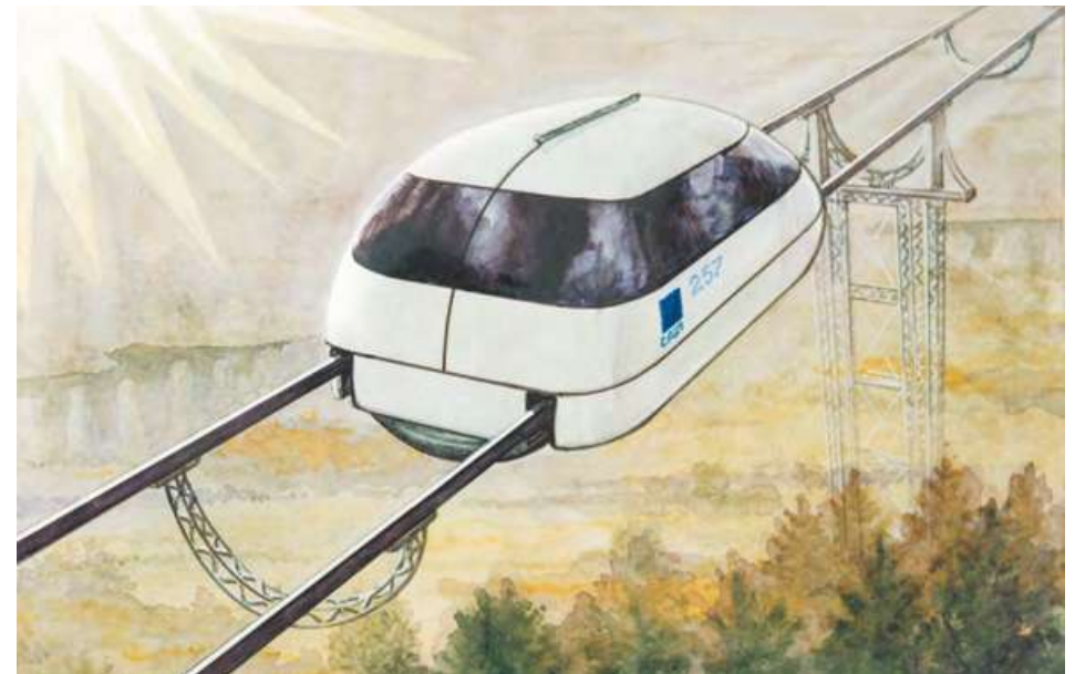
Figure 1.5 – NTL track on tower supports (about 100 m)
