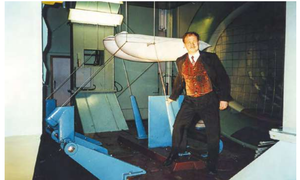
Wind-tunnel test of a double-body unibus model (scale 1 : 5). St. Petersburg, October 2000
