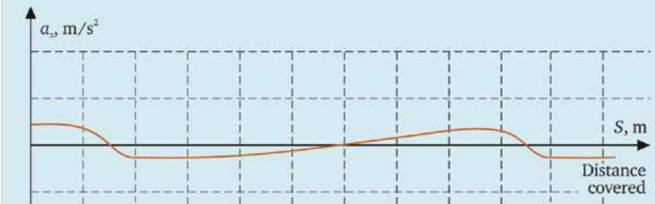
Diagram of vertical acceleration felt by passengers during movement
